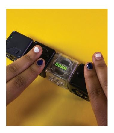
If your robot has two Sense blocks and one Action block, which one controls the robot? Build a Testbot with two Distance Sense blocks and a Bar Graph Action block between them.
