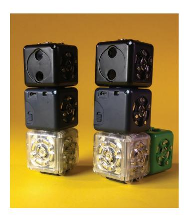
If you build this robot as a tower instead of a train, it still works, but it's no longer stable: approach the Distance Sense block and the Drive Action block starts moving. Accelerate too quickly and the tower falls over.
