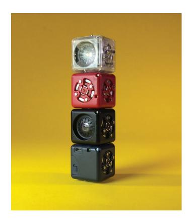
Put the red Inverse block between the Brightness Sense block and the Flashlight Action block. Remember the number flow story: every Sense block produces a number. The Brightness Sense block produces a big number when it senses a lot of light. It tells that big number to its neighbor (the Flashlight Action block), which turns the big number into a bright light.
