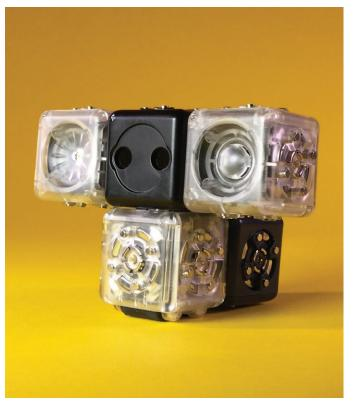
Build a simple Gobot with a Brightness Sense block and a Drive Action block: It goes when it senses light.
