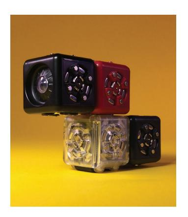
Swap out the Flashlight Action block and put a Drive Action block in its place. Now you've built a robot that goes when it's dark, and stops when it's light.
