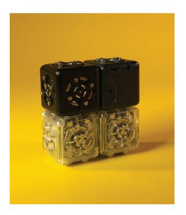
For example, make a robot and place the Brightness Sense block so its sensor face points down. Now it doesn't see the light. This Gobot is a Nogobot. No matter how bright the room is, the robot won't go. Its Brightness Sense block doesn't sense the light.
