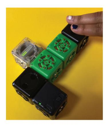
This robot shows the gradient story. The Bar Graph Action block is attached to one of two Passive blocks between two Distance Sense blocks, one at each end of the robot. The closer Distance Sense block has a bigger effect on the Bar Graph Action block. If your robot has an Action block right between two Sense blocks, the Action block averages the numbers the two Sense blocks tell it.
