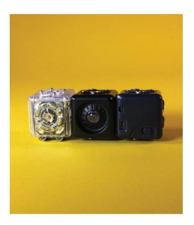
This simple brightness go-bot robot has a Drive Action block (left) that moves the robot when its Brightness Sense block sees light. The gray block on the right is the Battery block.
