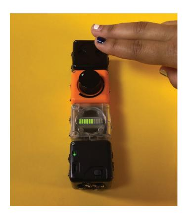
Construct a Testbot with a Battery, Bar Graph, and Distance Sensor. The closer an object is to the Distance Sensor, the higher the value displayed on the Bar Graph Cubelet.
