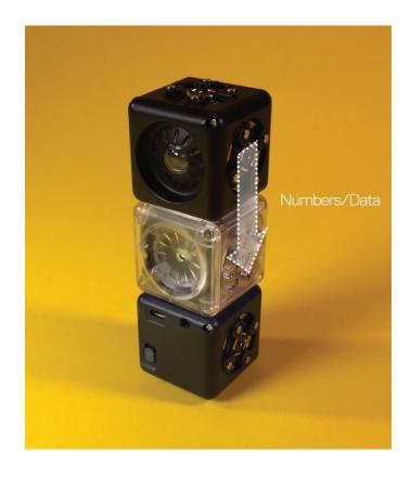
lamp dim. Think of the number as hopping or flowing from one block to the next. Numbers are flowing through the blocks of the robot from Sense blocks to Action blocks all the time. That's what makes the robot behave the way it does.
