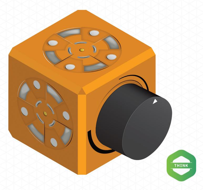
The Threshold Cubelet is a THINK Cubelet with an adjustable knob. It functions like a Blocker for an output values below the threshold you set. Output values that are above the threshold are pass along normally. Use the Threshold Cubelet to create robots that react suddenly, exhibit binary behavior, or gate SENSE outputs.
